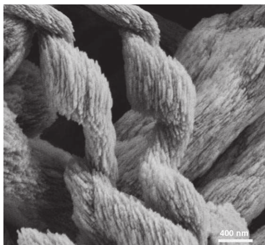
Figure 20. SEM image of helical BaCO 3 fibers formed in presence of a stiff phosphonated block copolymer. Reproduced from ref. [84] with permission of Nature Publishing Group.
