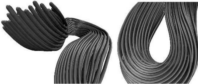
FIG. 13. Detailed view of a highly deformed CNT bundle under compressive load.
