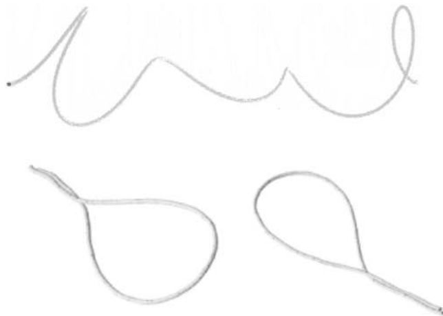
FIG. 1. Full atomistic calculations of the properties of ultralong CNTs as reported in Refs. 42 and 43. Above a critical aspect ratio, CNTs self-fold into racket-like structures. It can be observed that the self-aligned part connects to the free length of the CNT in a characteristic way by crossing over at an angle of around 90^\circ . We believe that this phenomenon could be explained due to the reduced energy by increasing the contact length in this characteristic manner.
