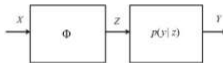
Figure.12: Generalized CS estimation problem. Here X \in \mathbb{R}^N is the vector to be estimated. Z \in \mathbb{R}^n is the measurements and Y \in \mathbb{R}^n is the noisy measurements.
