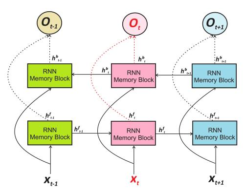
Figure 3. Typical Structure of Bidirectional Recurrent Neural Network shown at step three.
