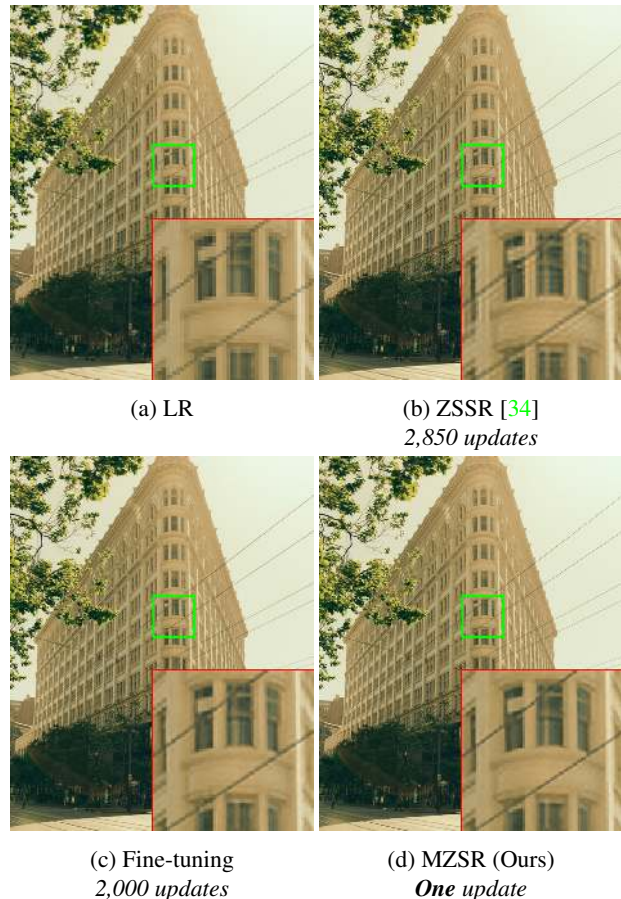
Figure 1: Super-resolved results ( \times 2 ) of “img050” in Urban100 [14]. The blur kernel of the LR image is an isotropic Gaussian kernel with width 2.0. Result of (c) is fine-tuned from a pre-trained model. Our MZSR outperforms other methods within just one single gradient descent update.
