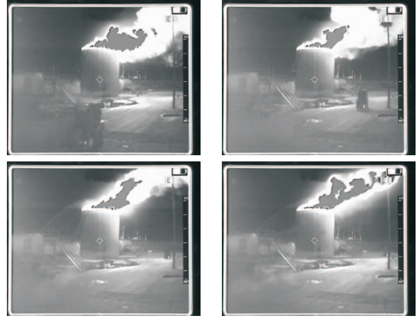
Fig. 9. Consecutive frames from a thermal video to detect fire presence.
