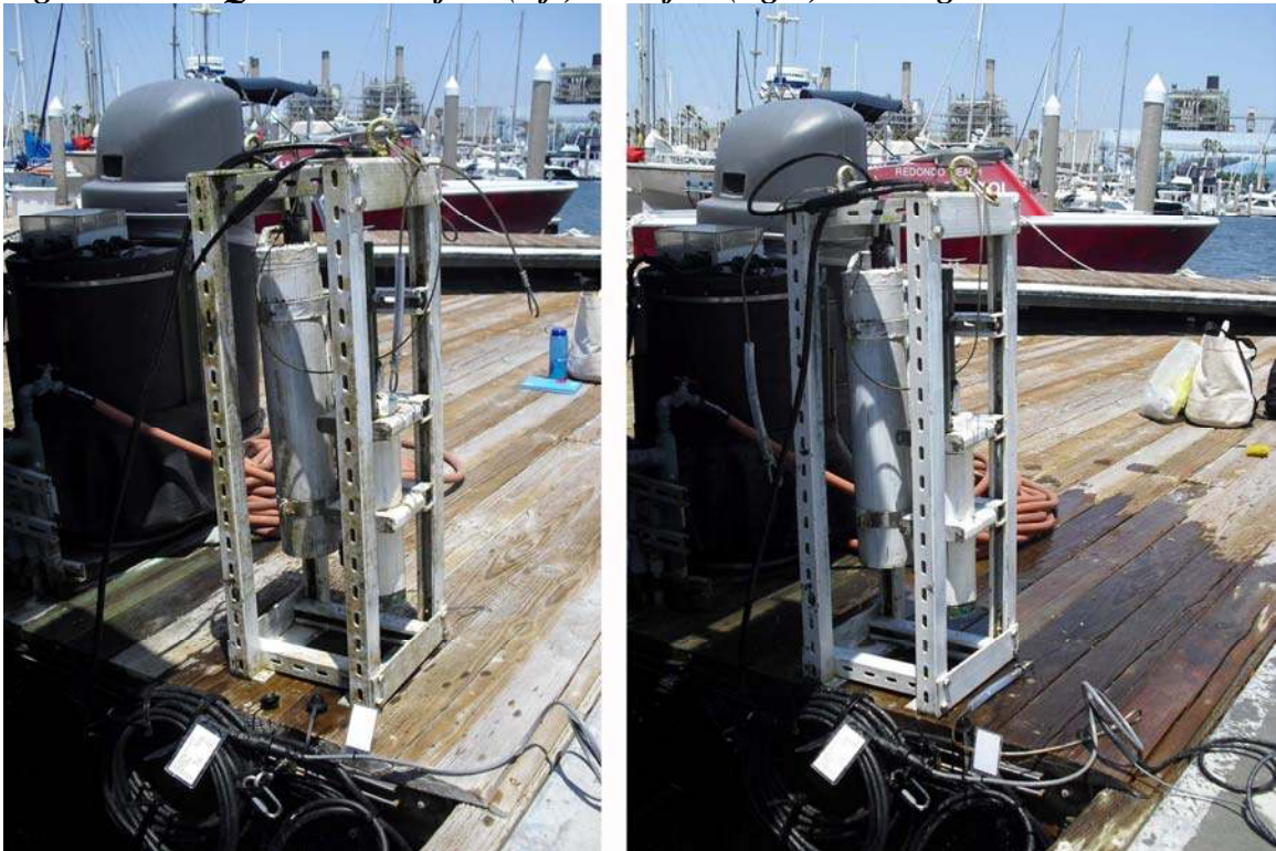
Figure 5.7 – WQM sensors before (left) and after (right) cleaning
