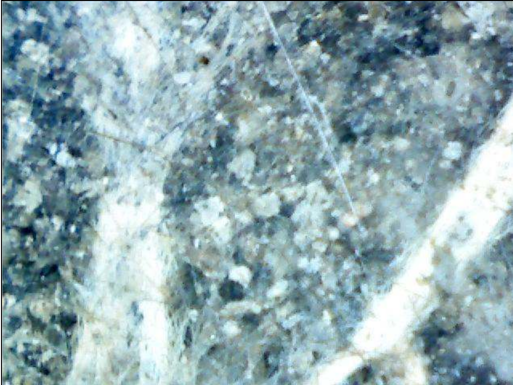
Figure 5.11 – Image taken by automated soil imaging system. The thick white lines illustrate roots passing through the image.
