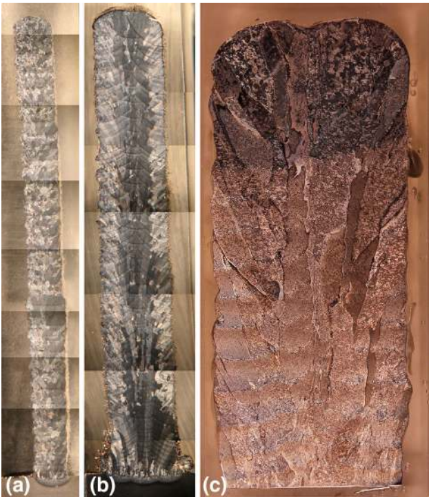
Fig. 5 Macro-graphic images of additive manufacture Ti-6Al-4V: (a) laser powder blown single bead wide, (b) laser powder blown three bead wide, and (c) electron beam wire three bead wide
