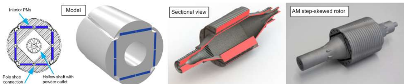
Figure 9. AM interior magnet-skewed rotor for PM synchronous machine with hollow shaft and lightweight construction [30].
