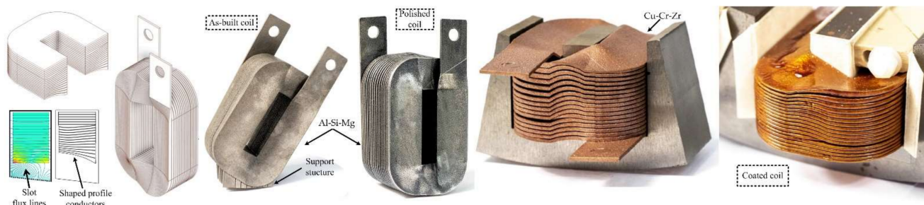
Figure 13. AM shaped-profile coils with low AC loss for high-speed electrical machines [39–41].
