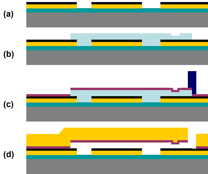
Figure 3. Switch process flow. (a) Deposition and patterning of bottom electrode and bottom contact metal. (b) Deposition and patterning of sacrificial layer with a small recess area for contact dimple formation. (c) Deposition of top metal contact metal which also serves as plating seed layer. Deposition and patterning of thick plating mold resist. (d) Plating cantilever beam, etching of excess seed layer and removing sacrificial layer to release the beam.
