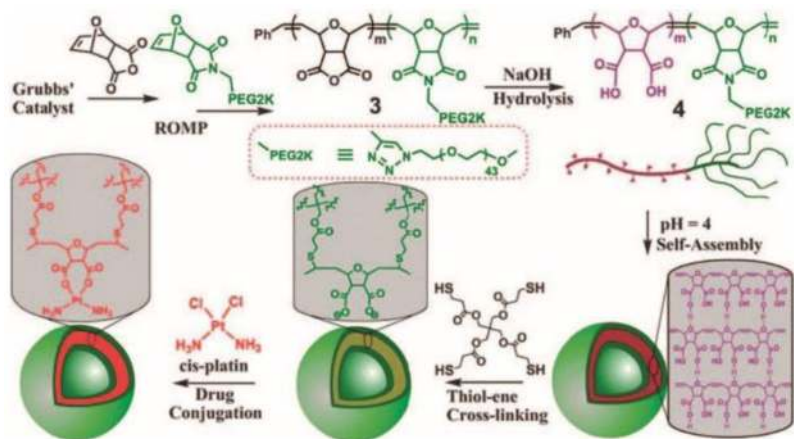
Fig. 30. Chemistry of constructing cross-linked polymer vesicles and their drug conjugation with cisplatin. Adapted with permission from Ref. 197. Copyright © 2012, Royal Society of Chemistry.
