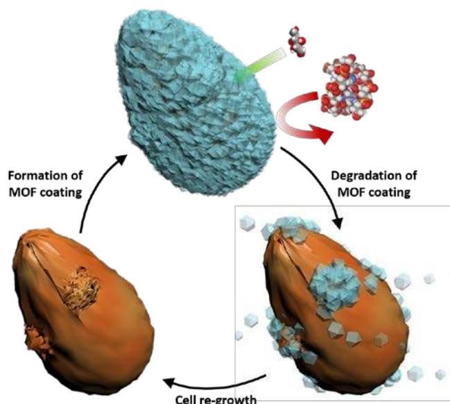
**Scheme 1.** Schematic illustration of biomimetic crystallization of cytoprotective metal-organic framework coatings on living cells.
