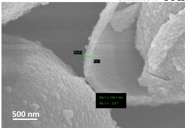
**Figure S5.** Cross-sectional SEM image of a cracked ZIF-8 shell on yeast showing the thickness of the ZIF-8 coating.
