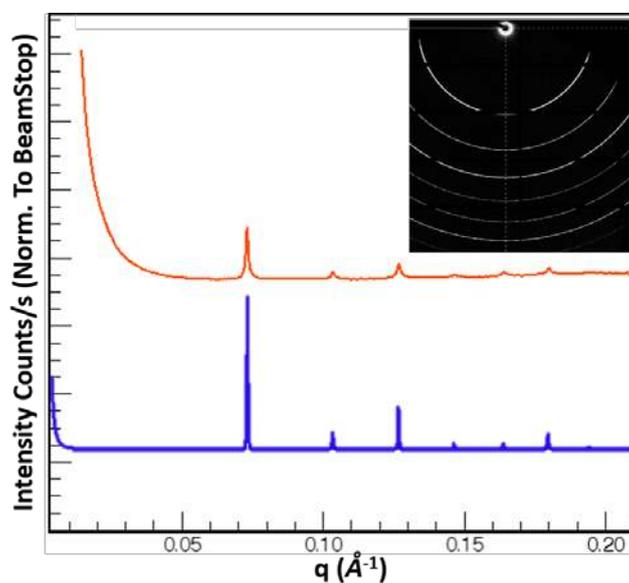
**Figure S4.** Synchrotron small-angle X-ray scattering (SAXS) diffraction patterns of standard ZIF-8 crystals (blue) and ZIF-8 coated yeast cells (red). Inset: 2D SAXS pattern of the ZIF-8 coated yeast cells (measure using a 0.5 mm capillary as a sample holder).
