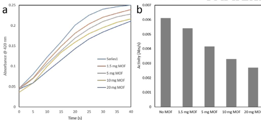
**Figure S11.** (a) Glucose oxidase-horseradish peroxidase coupled enzyme activity assay and (b) the initial gradient as a measurement of the amount of glucose.
