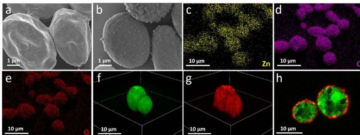
**Figure 1.** SEM images of (a) native yeast and (b) ZIF-8 coated yeast. (c-e) EDS elemental mappings of ZIF-8 coated yeast. 3D cellular reconstruction of CLSM images of ZIF-8 coated yeast cells (f-g), and (h) cellular cross-section. The living yeast cells were labelled with FDA (green) and the ZIF-8 coatings were labelled by infiltration of Alexa Fluor 647 fluorescent dyes (red).
