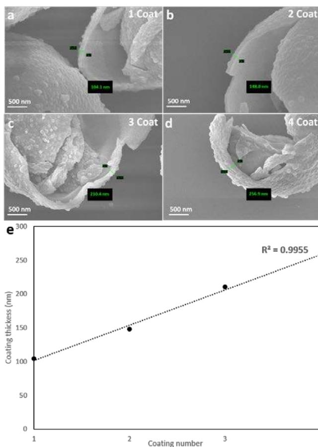
**Figure S6.** Cross-sectional SEM images of a cracked ZIF-8 shell on yeast. The SEM was used to measure the thickness of ZIF-8 coatings from 1 to 4 coating cycles. (a) 1 coating cycle, (b) 2 coating cycles, (c) 3 coating cycles, (d) 4 coating cycles. (e) Plot showing the corresponding ZIF-8 coating thickness with number of subsequent coating cycles.
