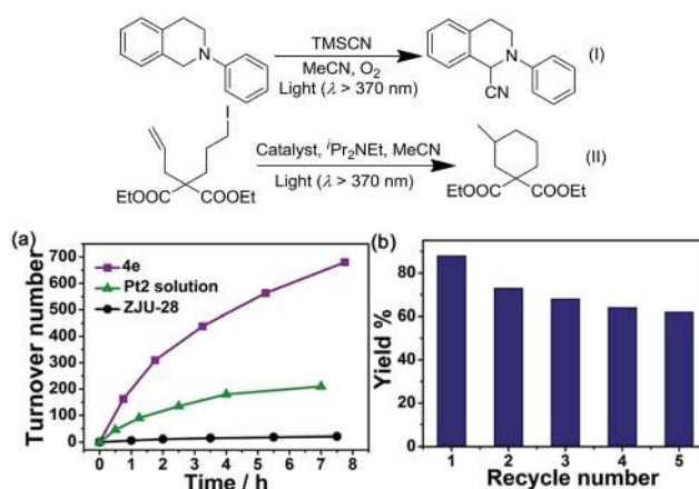
Fig. 5 (Top) Scheme of oxidative cyanation of a tertiary amine (I) and reductive cyclization of an alkyl iodide (II). (Bottom) (a) The time course of the oxidative cyanation by 4e (Pt 2 @ZJU-28), Pt 2 and ZJU-28; (b) the yield of the reaction in recycling experiments using 4e as the catalyst.
