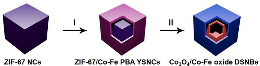
Figure 1. Schematic illustration of the formation process of Co 3 O 4 /Co-Fe oxide DSNBs: I) ion-exchange reaction between ZIF-67 NCs and [Fe(CN) 6 ] 3- ions to form ZIF-67/Co-Fe PBA YSNCs and II) subsequent conversion to the Co 3 O 4 /Co-Fe oxide DSNBs by thermal annealing.
