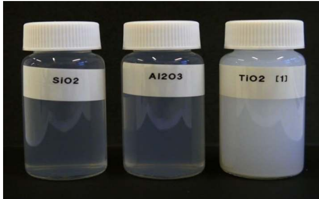
Fig. 4 Brine (NaCl 3 wt %) containing nanoparticles 0.05 wt % at initial condition
