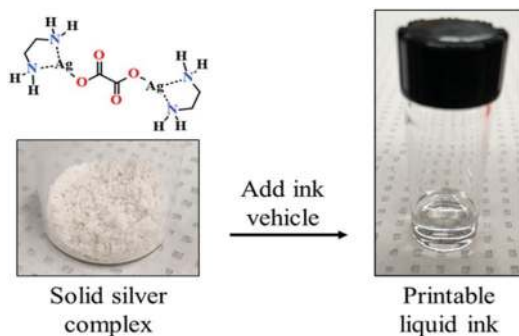
Fig. 18 Solid silver complex that can be converted to a desired printable liquid ink. Reproduced with permission from ref. 99. Copyright 2018, American Chemical Society.
