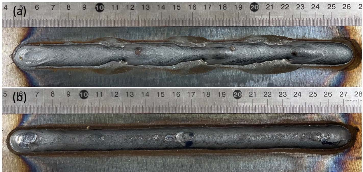
Figure 9. Weld bead appearance of solid wire (a) and metal-cored wire (b) at 280 A welding current.
