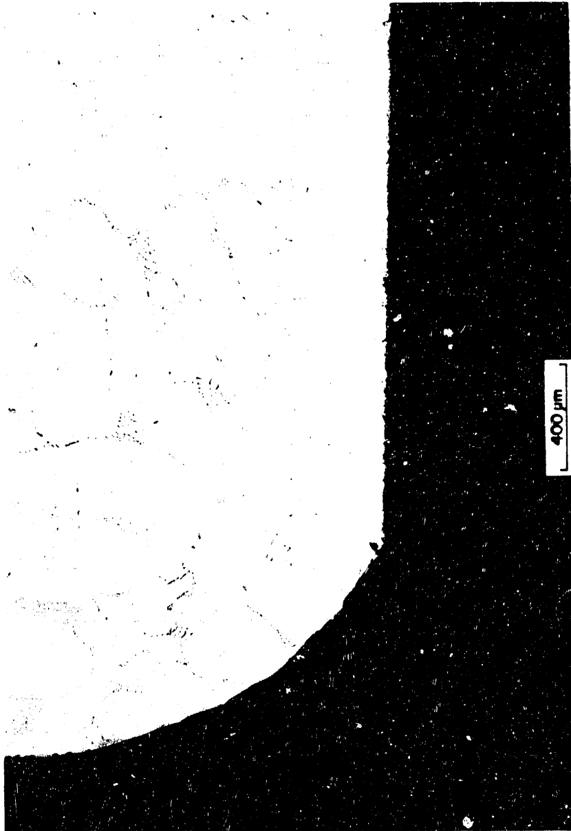
Fig. 4. Sessile drop of Ge-0.5% Ti alloy on a spectroscopic carbon planchette. Wetting angle \theta \approx 150^\circ .
