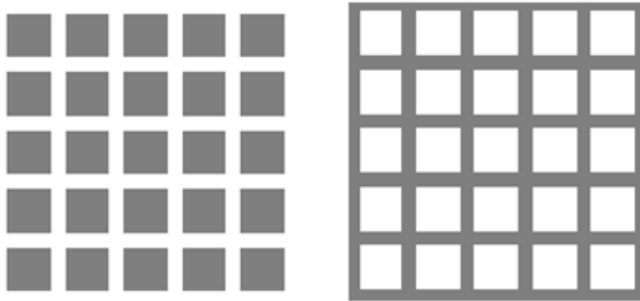
Fig. 3.4 – Basic FSS geometries: The patch-array produces a capacitive response, whereas the array of slots is inductive.
