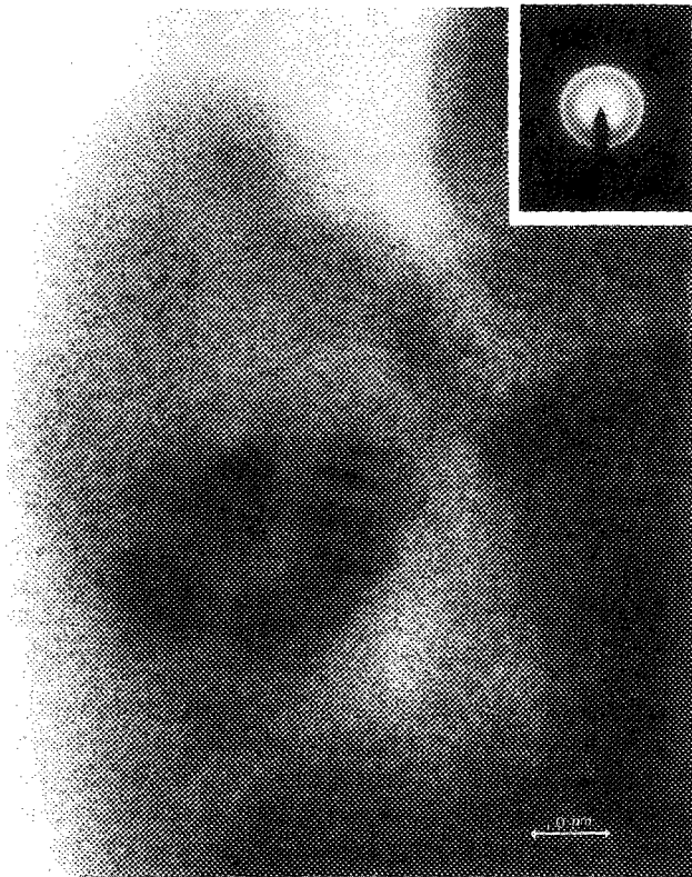
FIG. 3. TEM bright-field image of the amorphous Zr_{0.75}Al_{0.25} phase obtained after 12-h ball milling. The inset shows the corresponding diffraction pattern.
