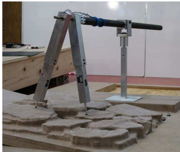
Fig. 25. Compass gait robot posed on rough terrain.
