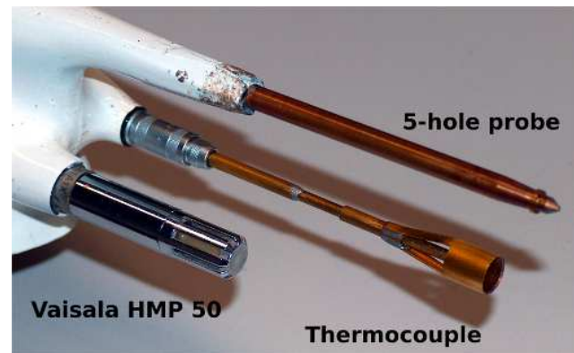
Fig. 2. The meteorological sensors of the M 2 AV.
