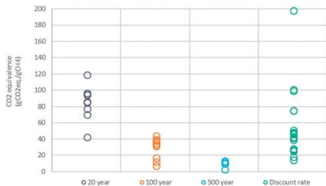
Fig. 7 CO 2 equivalence of methane for different time horizons and compared to metrics which use discount rates instead of time horizons.
