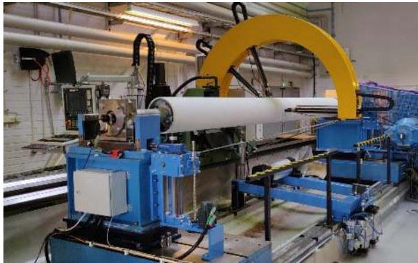
Fig. 7. Complete test setup. The accelerometers and force sensors were placed at the rotor ends, and displacement measurement was performed with laser sensors attached to the yellow arc
