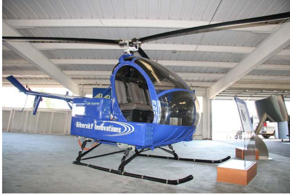
Figure 4: Sikorsky Firefly all-electric helicopter concept. This prototype shows similarity with a conventional helicopter as the main engine was directly replaced with an electric motor of the same power curve [144].
