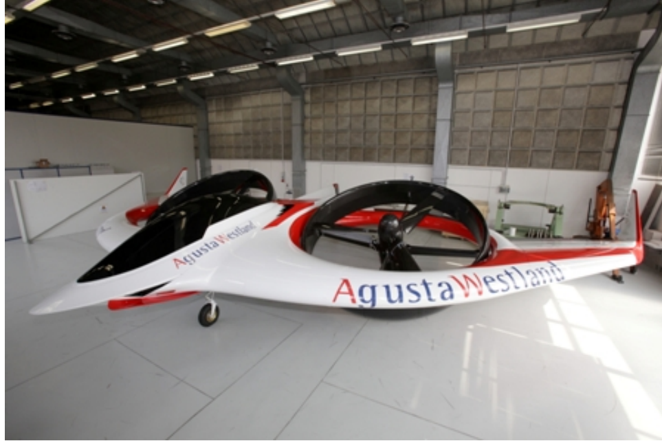
Figure 7: AgustaWestland Project Zero all-electric VTOL concept. The lift is generated with two ducted fans embedded in the wing during hover [4]. Both fans rotate during forward flight.
