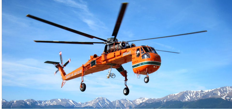
Figure 2: S-64E in flight, one of the most popular sky crane in use today. The unusual fuselage shape allows larger payload to be carried.
