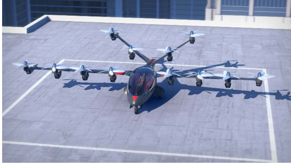
Figure 6: Joby S2 VTOL concept. 12 tilting motors are used to provide lift in hover, while two tip-mounted motors are used to provide thrust in cruise [151].
