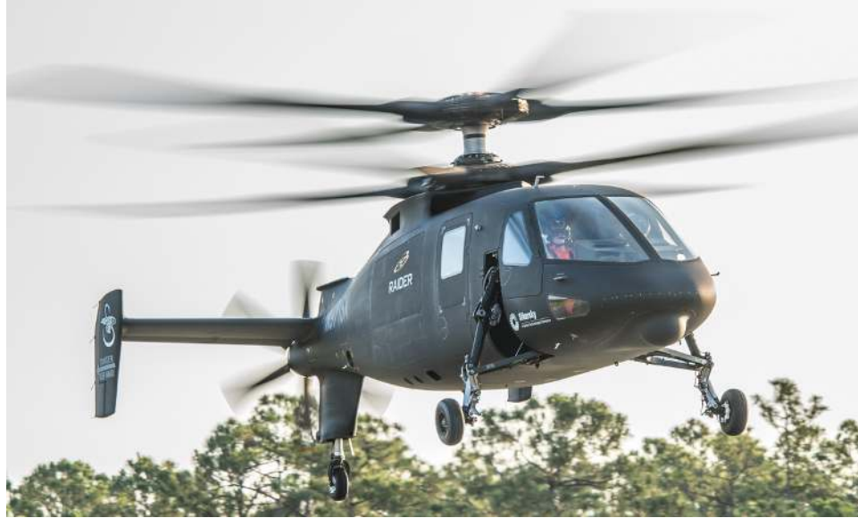
Figure 106: Sikorsky S-97 RAIDER. The coaxial configuration with load transfer on the advancing blade and a multibladed pusher propeller configuration allows for flight speeds on the order of 250 kts, but the fuel burn remains very high.
