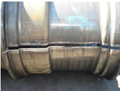
Fig. 7: Breaking of the workpiece basic material.
