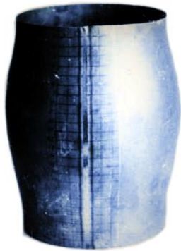
Fig. 14: Cylindrical sample after stamping.
