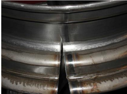
Fig. 5: The weld zone rupture in the wheel rim.
