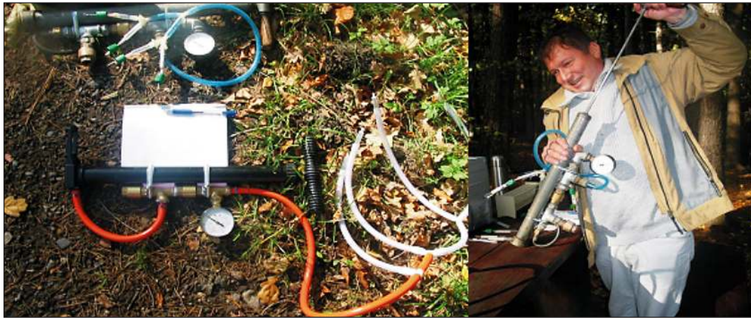
Fig. 2. After sampling the leave rings were placed in test tubes and exposed to low pressure treatment (0.33 atm.). The manual low pressure system is constructed with two valves, vacuumeter and pump with conversed piston
