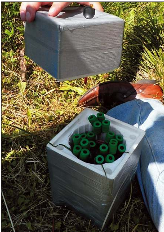
Fig. 3. Temperature in incubation chamber is stable, it is filled with water and allow for fast adjust of temperature. The temperature is set and adjust to constant level for all incubation time using ice cubes or warm water
