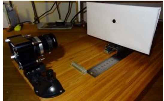
Fig. 2. View of the measuring system. Marker diameter is 0.01 m.
