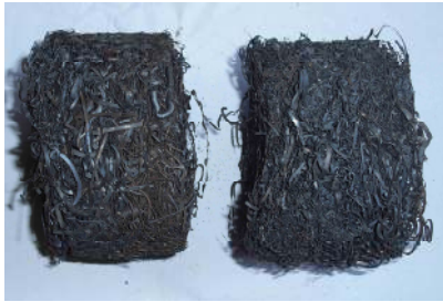
Fig. 1. Annealed and compacted billet of steel waste chips as desulfurizer
