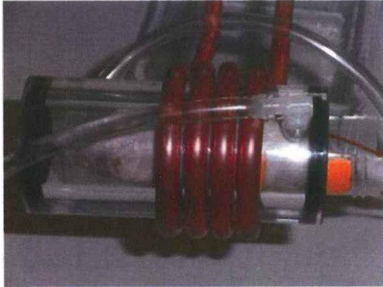
Figure 3. Picture of the 4-turn solenoid coil, water jacket and mouse chamber with anaesthetised mouse inside.
