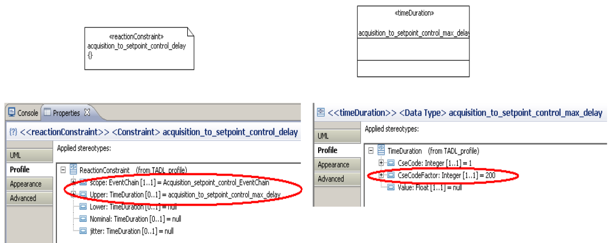
Figure 31b Specification of the timing constraint for the acquisition setpoint control event chain
