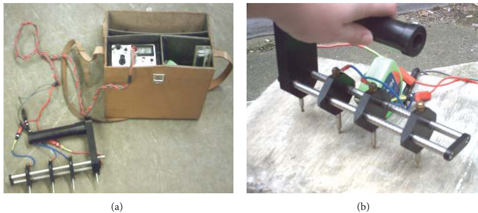
FIGURE 5: Concrete resistivity measurement: (a) test setup and (b) measurement.
