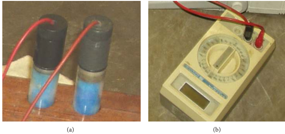
FIGURE 4: Half-cell potential measurements: (a) copper/copper sulphate electrode and (b) digital voltmeter.
