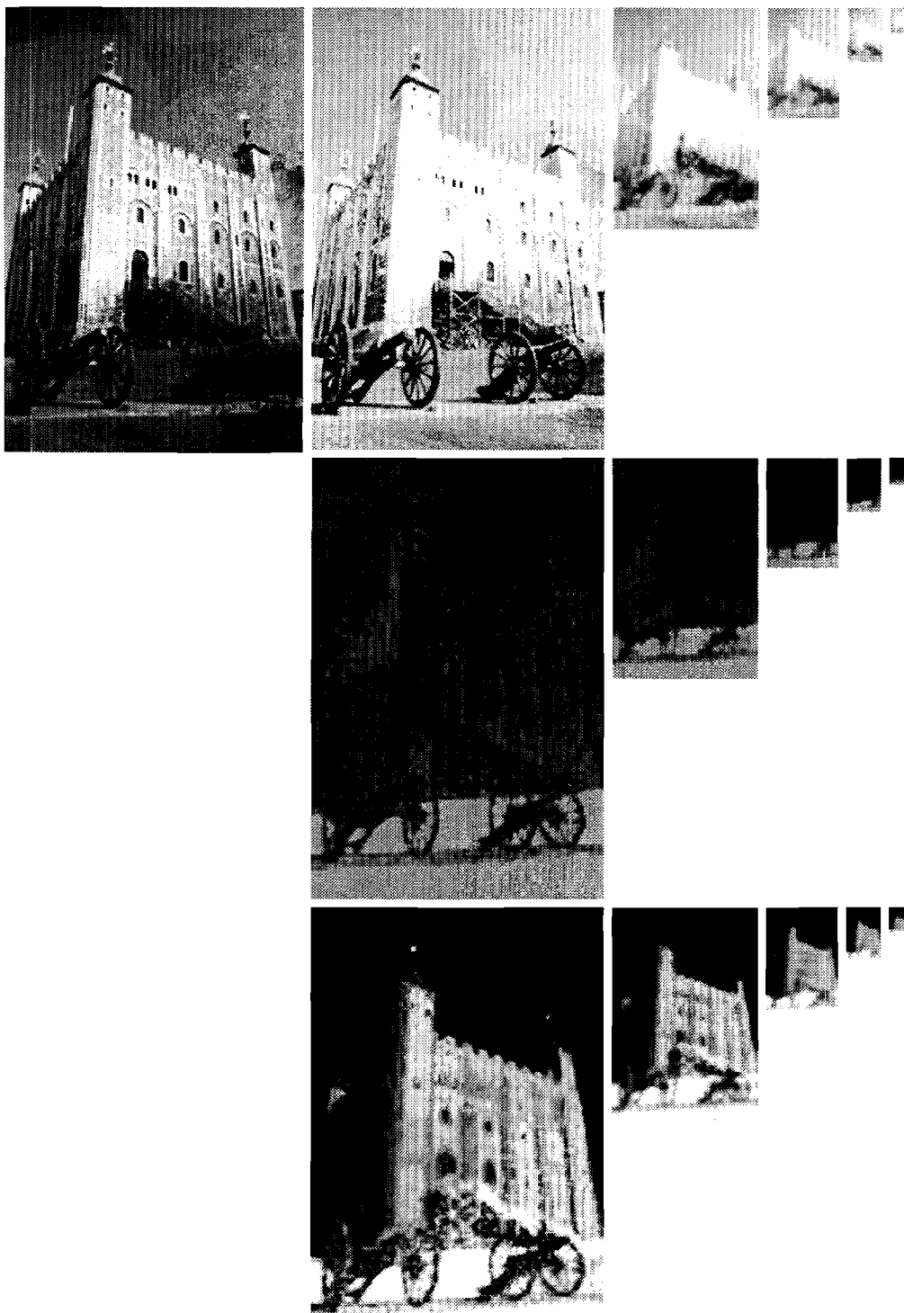
Figure 13: Gaussian pyramid decomposition. The figure shows the Lab pyramid decomposition of the color image in the upper left corner. From top to bottom, the rows contain the pyramids for the L^* , a^* and b^* channels.
