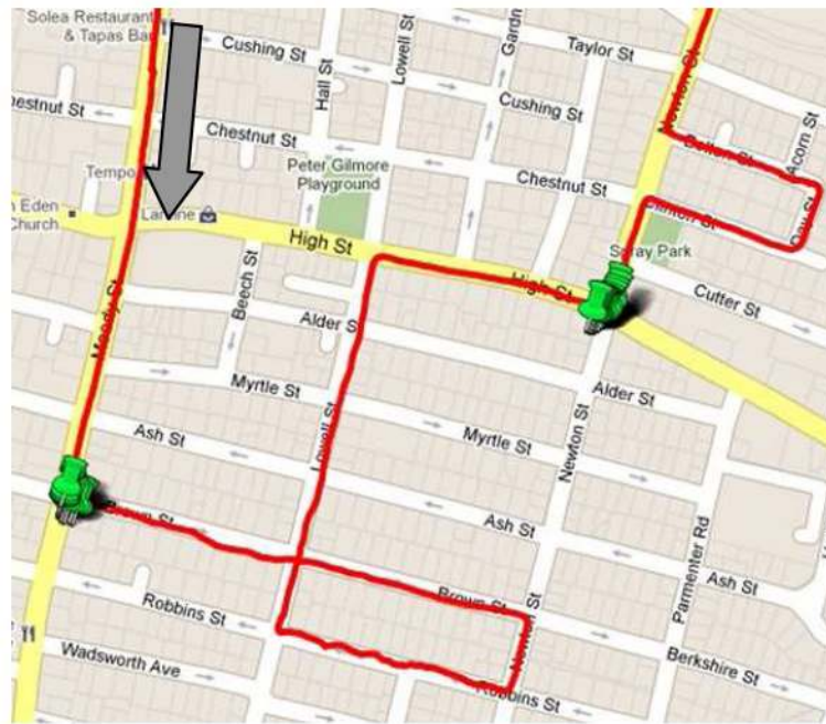
Figure 5. Detection of left turns on major roads (shown in yellow) by filtering left turn detection results with road class data at intersections. Note that the two left turns at minor intersections are not flagged, nor are the right turns.
