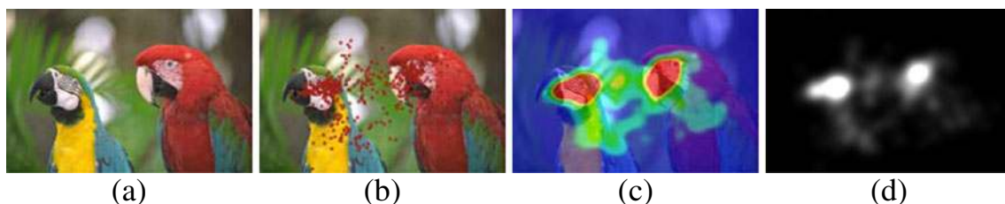
Fig. 3 From left to right: a original, b fixation map with red fixation points, c heat map (red spots represent the most visually salient areas of the picture), and d saliency map
