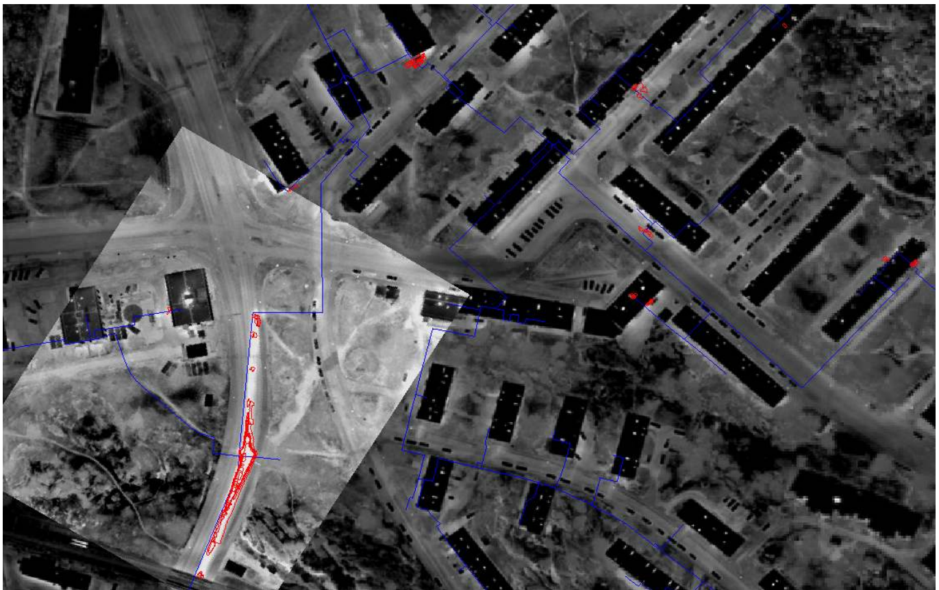
Fig. 8. Another detection example over a larger area visualized as an image mosaic. Candidate detections are shown in red and district heating pipes as blue lines. One major leakage is found in the image with a brighter color scale. A few false alarms are also present, typically around buildings.
