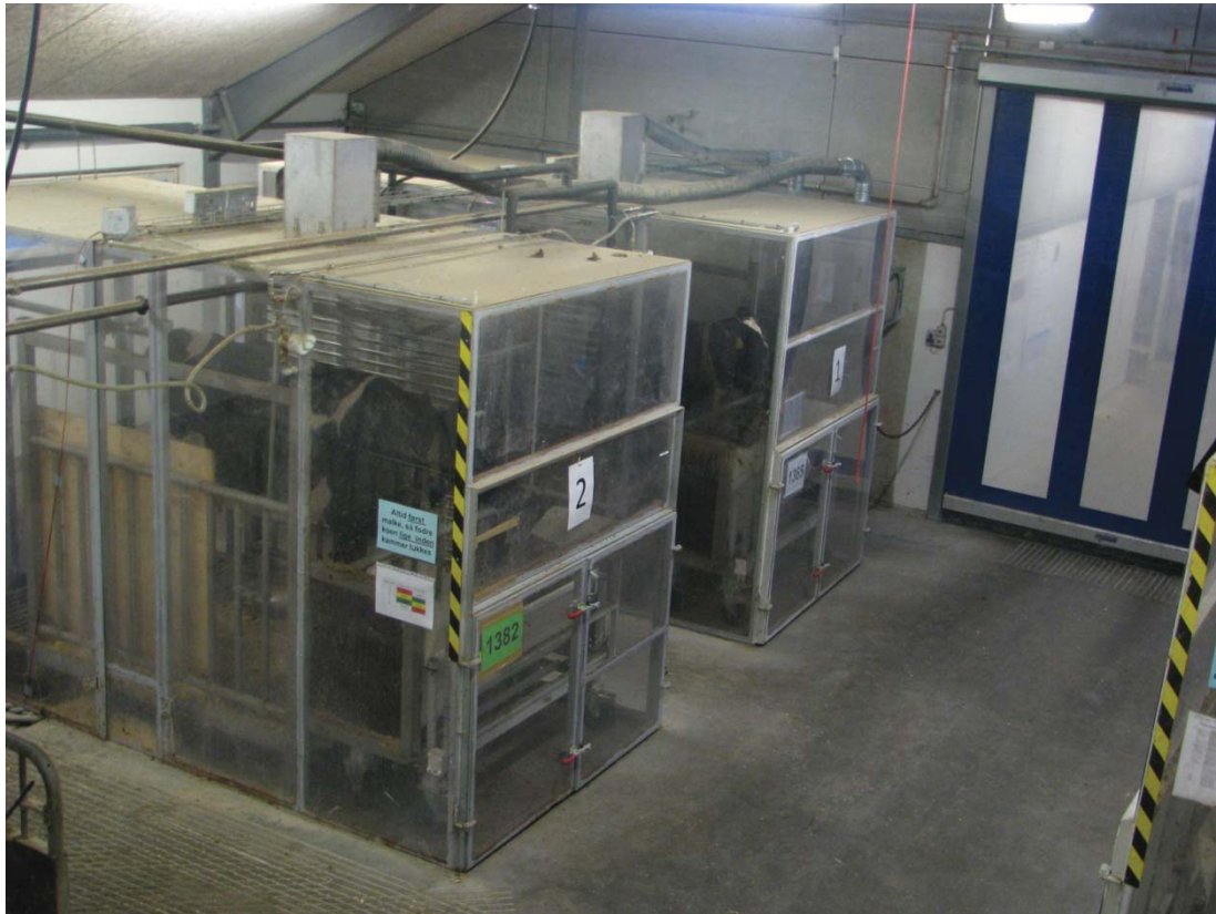
Figure 2. Respiration chambers constructed at Aarhus University of a steel frame covered with polycarbonate.
