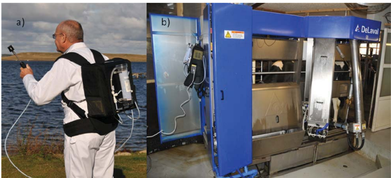
Figure 5. The portable Gaset (a) used for measuring CH 4 and CO 2 concentrations in an automated milking system (b).
