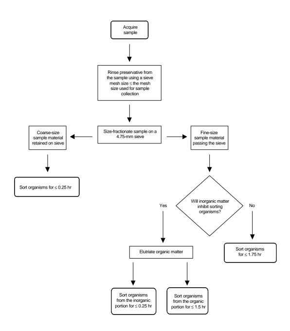
**Figure 4.** Overview of the qualitative, visual sort method for processing benthic macroinvertebrate samples. mm, millimeter; hr, hour(s); =, less than or equal to.
