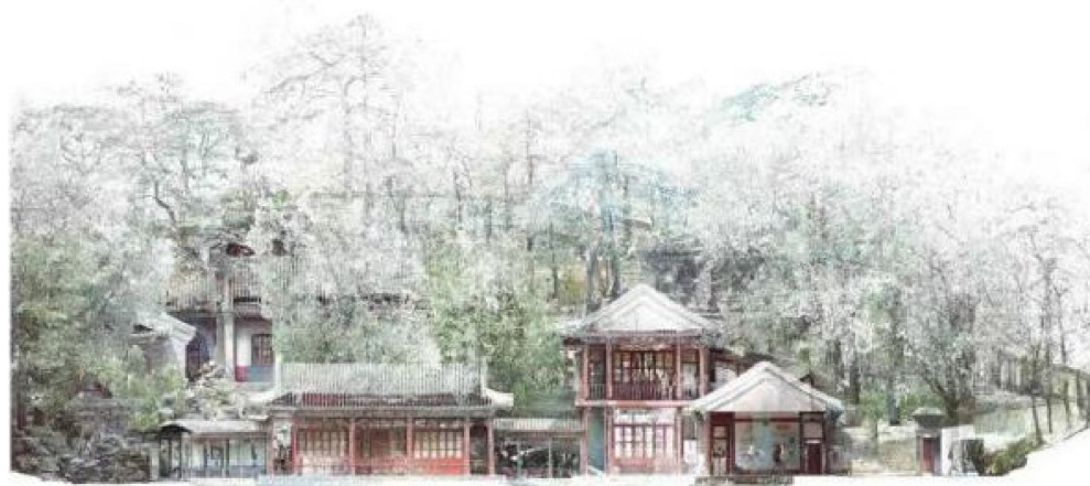
Figure 6. Garden-wide orthogonal maps from the point cloud model of the Jianxin Courtyard.
