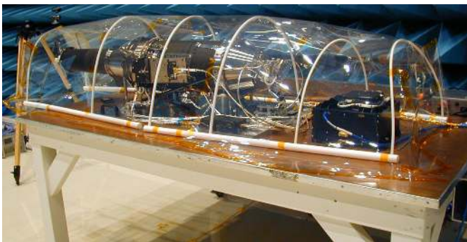
Fig. 28. Metis flight model during final electromagnetic cleanliness test at the ESA/ESTEC Test Center.
