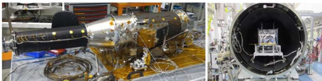
Fig. 25. Metis structural thermal model prepared for the vacuum thermal-balance test with temperature sensors installed inside and on the external surface ( left ). Metis structural thermal model inside the thermal-vacuum chamber endowed with Sun simulator, at ESTEC/ESA ( right ).
