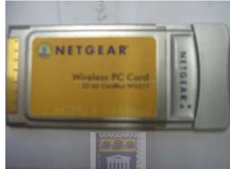
Figure 18: The Netgear wireless PC card used in the PC
