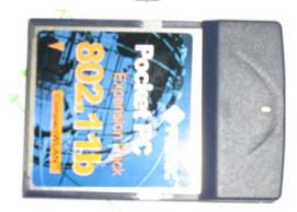
Figure 19: The Pretec pocket PC CompactWLAN used in the iPAQ h3870
