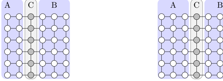
Figure 3: Two examples of conditioning to reduce the treewidth of a 6 \times 6 grid from 6 to 3.
