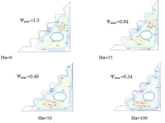
**Figure 7.** Streamlines for Ra =  $10^5$ , w = 0, and  $\phi$  = 0.02.
