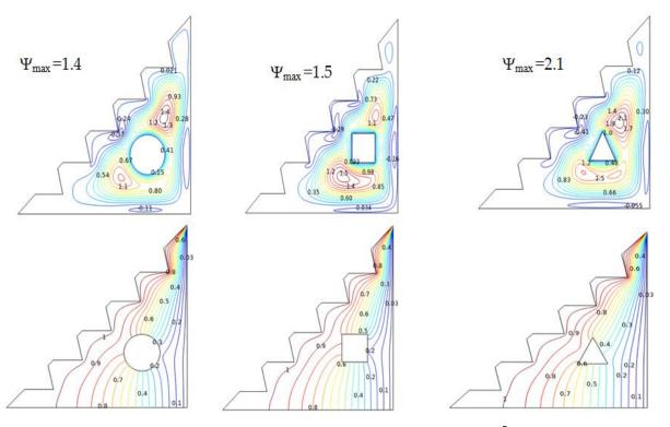
**Figure 10.** Streamlines and isotherms for w = 0, Ha = 0,  $Ra = 10^5$ , and  $\phi = 0.02$ .
