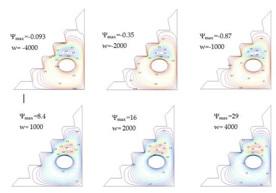
**Figure 9.** Streamlines via w and Ra =  $10^5$ ,  $\phi = 0.04$ , and Ha = 0.
