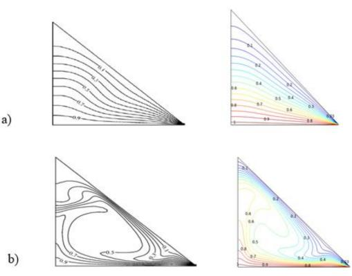
**Figure 3.** Isotherm and streamline comparison: previous work (left) and current work (right) for Ha = 0 (**a**),  $Ra = 10^4$  (**b**), and  $Ra = 10^6$ .
