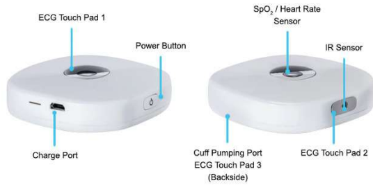
Fig. 4. Mintti Vision 6in1 health monitoring device [17]
