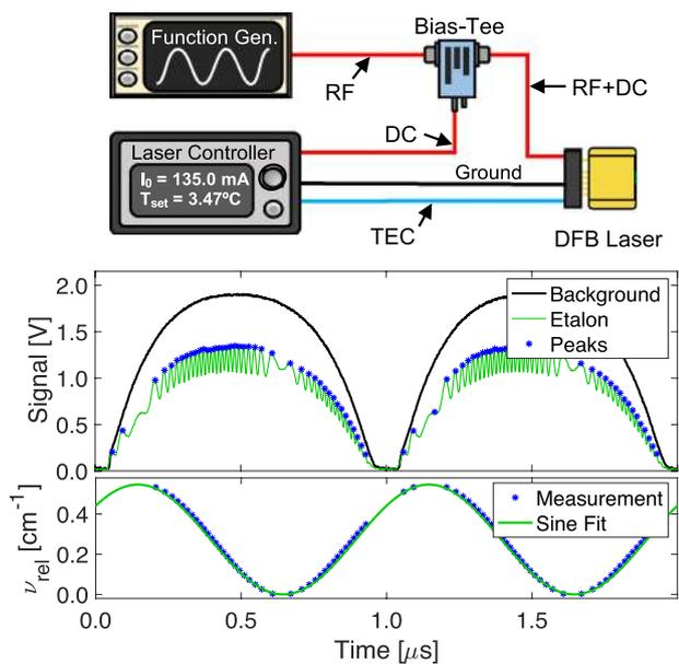
**Fig. 1** Bias-tee laser control schematic (top). Sample MHz laser scans showing background and etalon scans (middle). Plot of resulting relative wavenumber vs. time calculated from the etalon peaks with sinusoidal fit (bottom)
