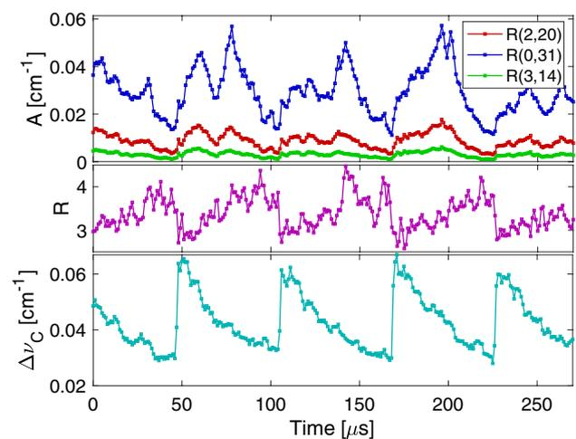
**Fig. 12** Time-resolved absorbance areas of the P(0,31), P(2,20) and P(3,14) lines of CO (top). The time-resolved ratio of absorbance areas of the P(0,31) and P(2,20) lines (middle). Time-resolved collisional-width (bottom)
