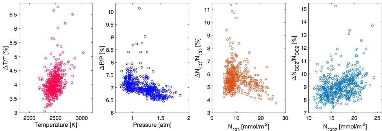
**Fig. 19** Relative experimental uncertainty distributions for temperature, CO and CO<sub>2</sub> column number density and pressure for the test shown in Fig. 16
