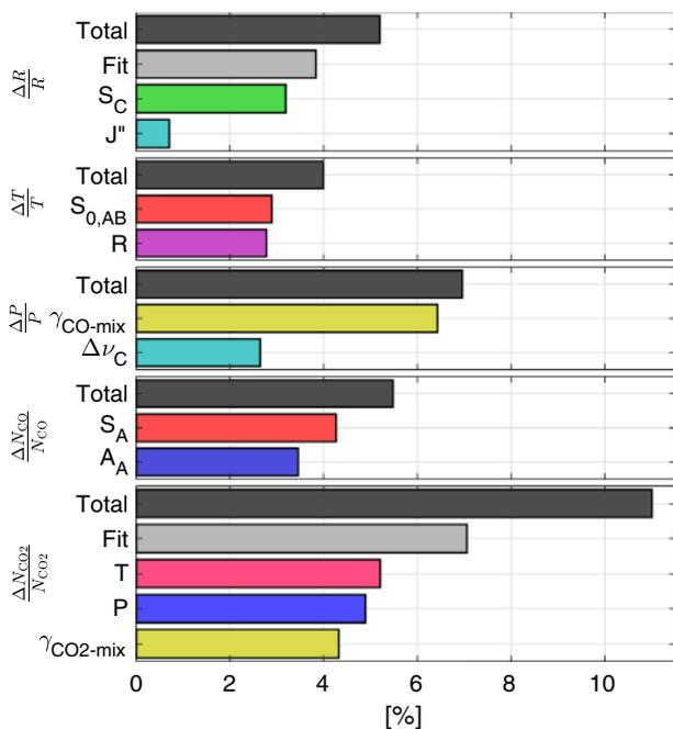
**Fig. 18** Representative uncertainties for linestrength ratio  $R$ , temperature  $T$ , column density  $N_{CO}$ , total pressure  $P_{tot}$ , and column density  $N_{CO_2}$  performed on the test shown in Fig. 16. Note: these values are averaged over a time series of measurements
