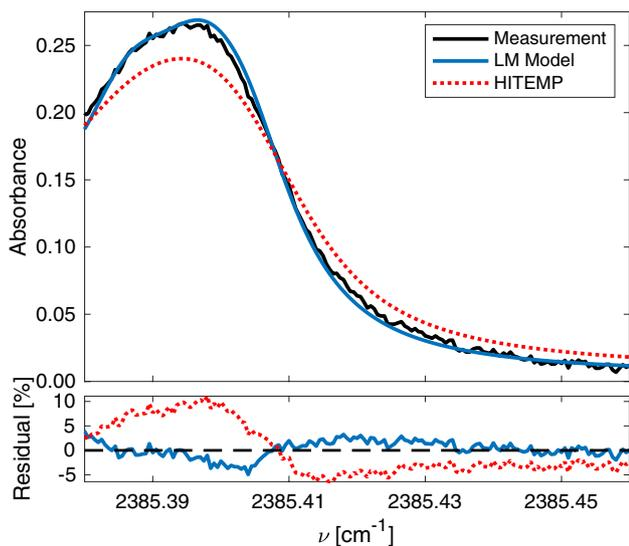
**Fig. 8** Absorbance for the targeted (01<sup>1</sup>0 → 01<sup>1</sup>1) bandhead of CO<sub>2</sub> in an Ar bath gas measured in the UCLA High-Enthalpy Shock Tube facility, alongside predictions with and without the line-mixing model implemented.  $X_{CO_2} = 0.03$ ,  $P_{tot} = 0.95$  atm,  $T = 2221$  K,  $L = 10.32$  cm
