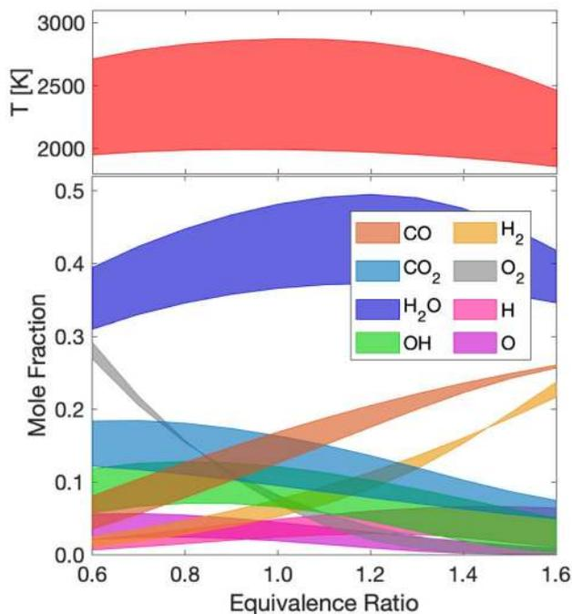
**Fig. 6** Plot of the temperature (top) and gas composition (bottom) for a CH<sub>4</sub>/O<sub>2</sub> detonation gas expanded isentropically to one atmosphere. Each quantity is plotted as a range to indicate the variation in gas properties between equilibrium and frozen flow
