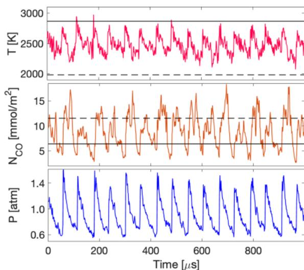
**Fig. 13** Time-resolved temperature (top), CO column density (middle) and pressure over 1000  $\mu\text{s}$ . The temperature and column density values predicted from CANTERA at  $P_{\text{tot}} = 1$  atm are shown for equilibrium flow as solid black curves and for frozen flow as dashed black curves. A path length of 1 cm is assumed for the column density
