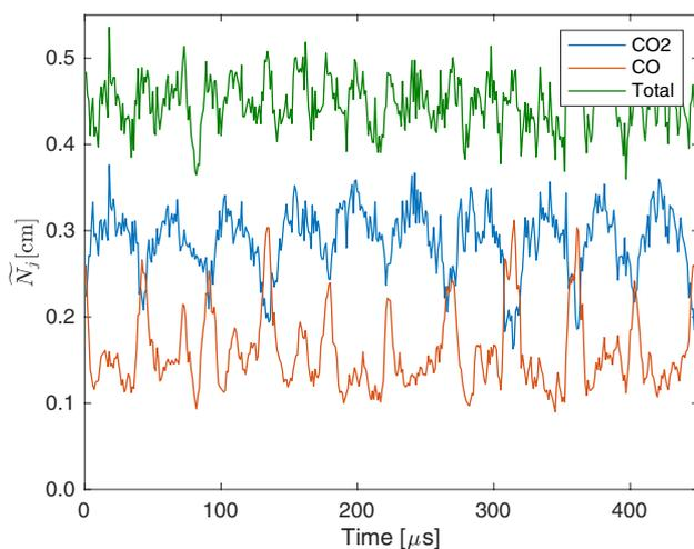
**Fig. 16** Time-resolved profiles of temperature and pressure normalized column number densities  $\tilde{N}_j$  for CO, CO<sub>2</sub>, and their sum
