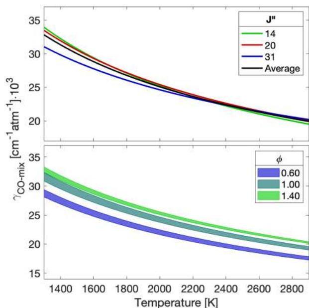
**Fig. 7**  $\gamma_{\text{CO}_2\text{-mix}}(T)$  plotted as a function of temperature for different rovibrational transitions  $J''$  (top) as well as for different gas compositions corresponding to varying RDRE operation conditions and frozen vs. equilibrium assumptions (bottom)
