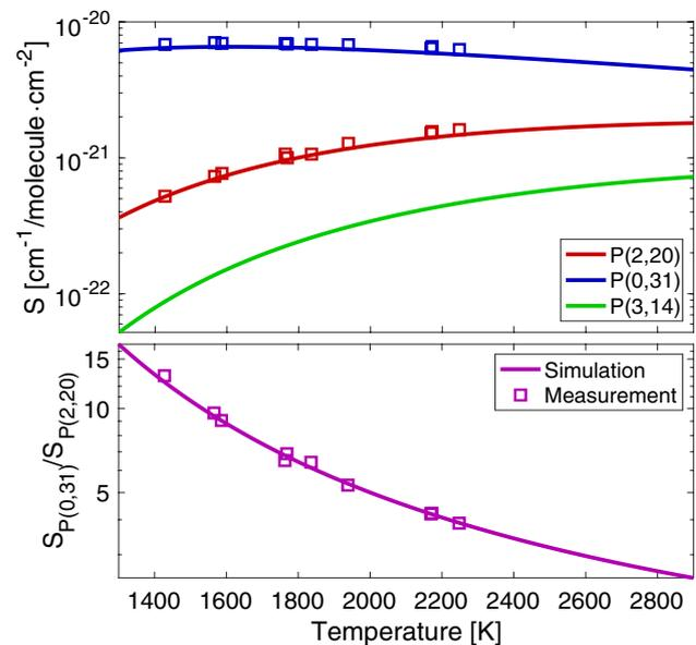
**Fig. 4** Linestrengths vs. temperature for the three target transitions. The ratio of linestrengths between the P(0,31) and P(2,20) line are also shown vs. temperature. Both simulated values of the linestrength ratio using the HITEMP database [38] and measurements from the UCLA High-Enthalpy Shock Tube facility are shown
