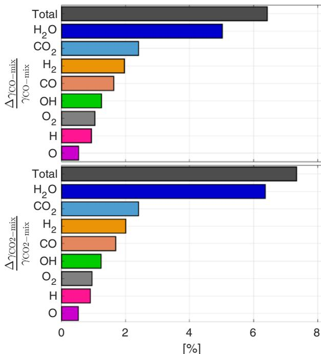
**Fig. 22** Averaged representative uncertainty analysis for the mixture-weighted broadening coefficients for CO and CO<sub>2</sub> performed on the test shown in Fig. 16
