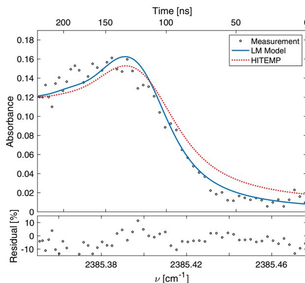
**Fig. 15** Example scanned-wavelength CO<sub>2</sub> bandhead data from the RDRE experiments, showing an effective measurement integration time of 250 ns
