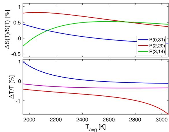
**Fig. 20** The relative difference between  $\overline{S(T)}$  and  $S(\bar{T})$  for the P(0,31), P(2,20) and P(3,14) (top) and the difference between  $\bar{T}$  and the temperature inferred from the  $\overline{S}$  for the P(0,31) line (blue), the P(2,20) line (red) and from their ratio (purple)
