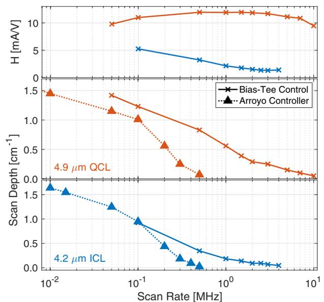
**Fig. 2** Plot of voltage-to-current transfer function versus scan frequency for the bias-tee circuits (top). Plot of scan depth vs. scan frequency with and without bias-tee control for both the QCL and ICL (bottom)
