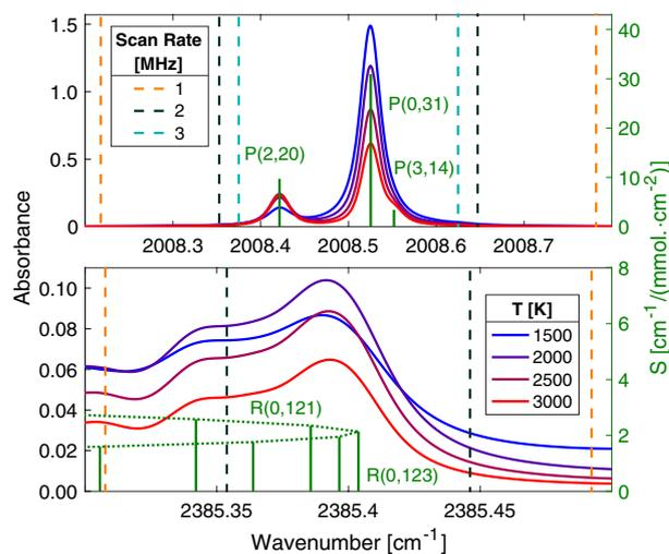
**Fig. 3** Target CO and CO<sub>2</sub> absorption spectra at relevant temperatures for  $X_{\text{CO}} = 0.20$ ,  $X_{\text{CO}_2} = 0.15$ , atmospheric pressure, and a 1 cm optical path-length. Linestrengths for the target transitions are plotted overlaid at 2500 K
