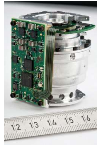
Fig. 8. One of three motor modules (metric scale ruler)
