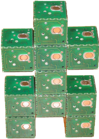
Fig. 15. The final robot-like shape we “self-disassembled” using an initial 3-by-5 rectangle of modules. From start to finish, the self-disassembly process required a total of approximately 90 seconds excluding any time spent modeling the desired final shape.
