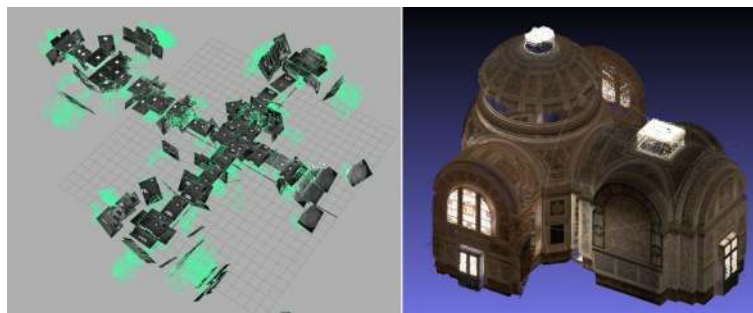
Fig. 7 Indoor architecture: Chapelle imperiale Ajaccio, with 100 fish-eye images; left : retrieved camera poses, right : 3D model
