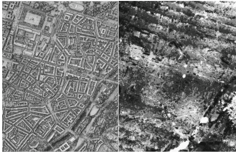
Fig. 6 Munich dataset, acquired with a DMC camera at GSD of 10 cm. Left : the depth map, right : the y-parallax generated with MMTestOrient . The amplitude of transverse parallax is \pm 0.1 pixel
