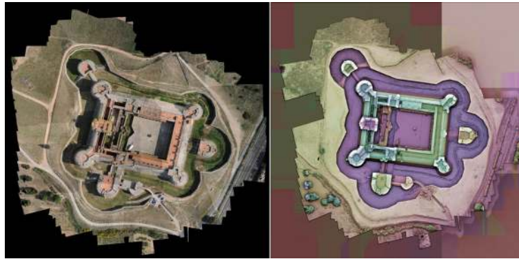
Fig. 8 Forteresse de Salses, photo acquired from a drone, in collaboration with Map-CNRS/ Left : hypsometry and shading maps overlapped, right : an orthophotography
