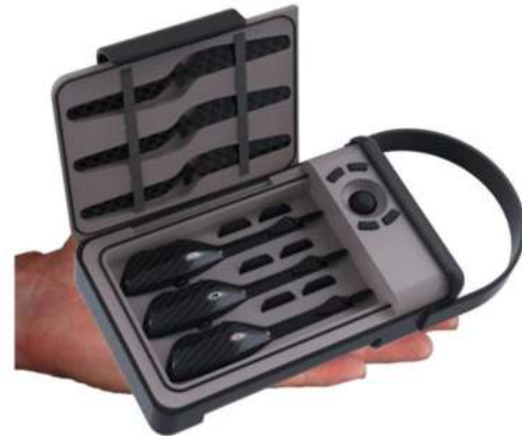
FIGURE 25: Graphic representation of the GCS from Prox Dynamics, containing three NAVs in the bottom side while the controls and the LED screen are placed on the upper side [17].
