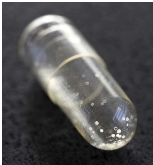
Figure 6.3: The image shows released micro containers collected in a capsule.
