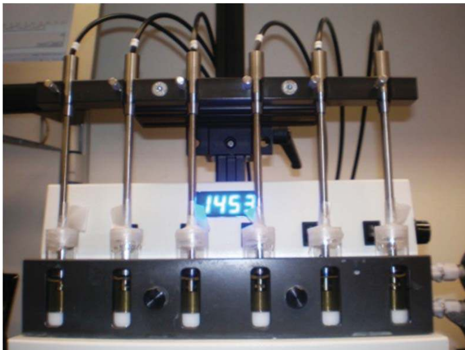
Figure 7.1: The image shows the Pion \mu DISS profiler used for dissolution experiments. It is seen that the machine has six separate testing setups consisting of a UV probe that is inserted in a beaker with solution. The beaker has a sample holder at the bottom which at the same time functions as a magnetic stirrer.
